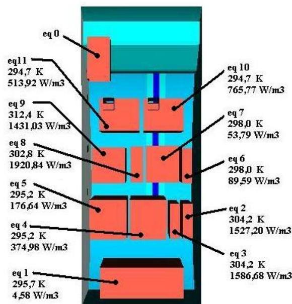
Figure 4. Experimental temperature values (K) and calculated heat generation (W/m<sup>3</sup>) for each device.
