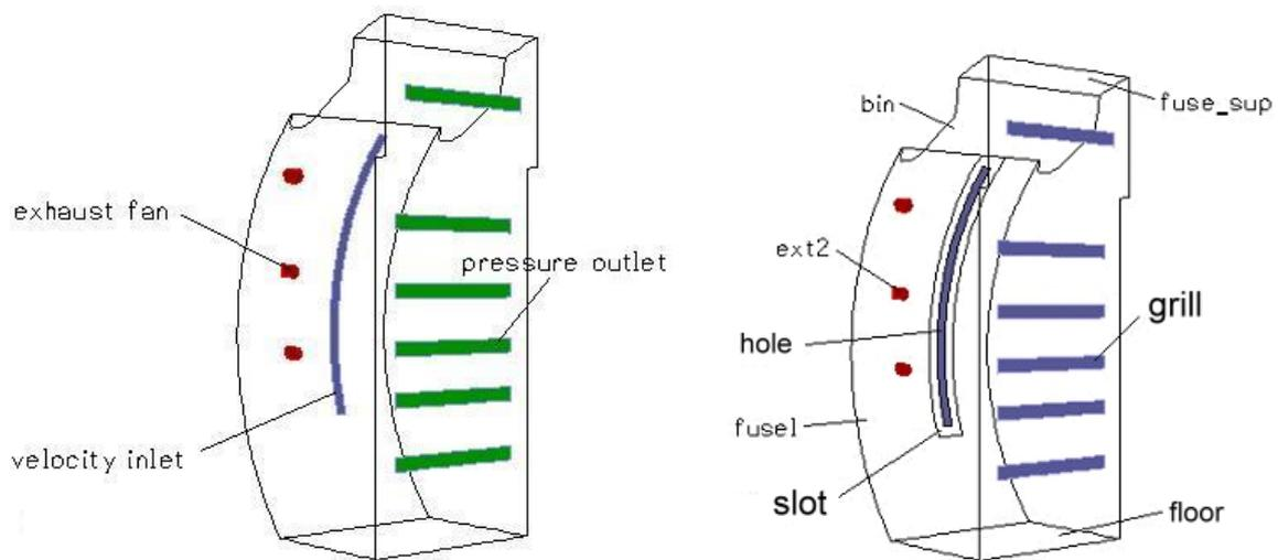
Figure 3. Representation of the rack boundary conditions.
