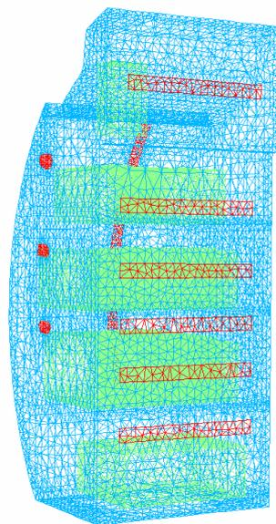
Figure 2. Mesh inside the rack with 93,503 tetrahedral elements.
