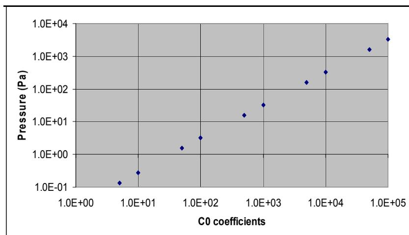
Figure 8. Relation between  $C_0$  coefficients and inlet pressure.
