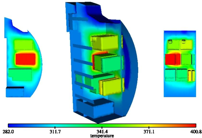
Figure 7. Temperature distribution (K) results for case without ventilation and without cables.
