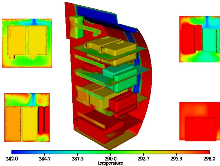
Figure 5a. Temperature distribution (K) results for the baseline case: transversal planes
